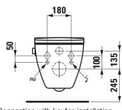
Connection with Laufen installation system LIS CW2
